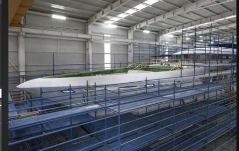
Over the years of experience and production, Sarp Yachts can offer internal and external service dedicated to yacht paint application: preparation, protection, treatment (sanding, fairing, cleaning) and finishing. Air temperatures are continuously controlled with other parameters such as hull temperature and air humidity, — is monitored and recorded to ensure a superb paint finish. A faultless finish demands rigorous initial conditions.
